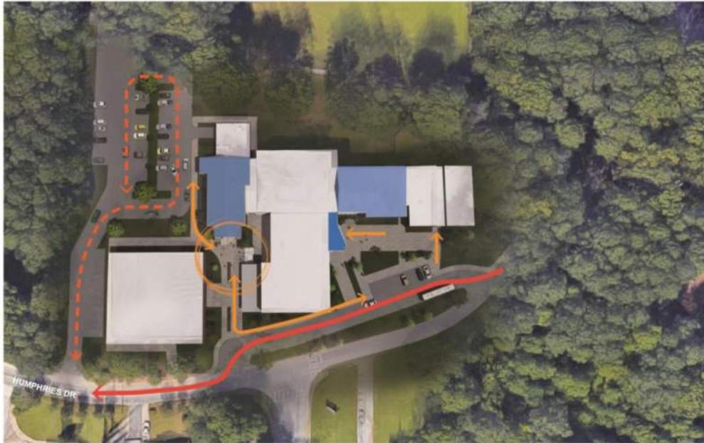
Site Plan of potential site traffic management upgrades (front bus loop and rear car rider drop off).
